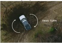
forward and some wheels backwards at the same time. This allows the truck to turn 360° like a tank. Other innovations include lots of storage space (because there's no gas engine taking up space) and a tailgate that folds down twice. How would you design a truck?
